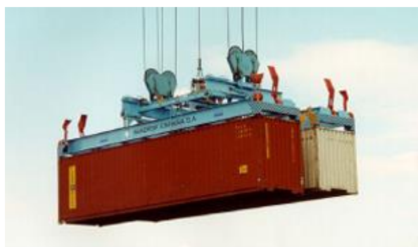
Obr. 1.11 Spreader se systémem tandem lift [21]
