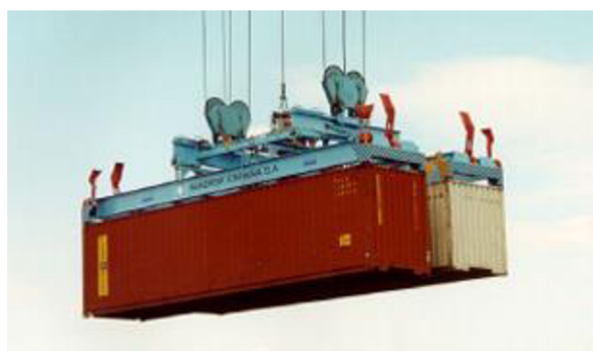
Obr. 1.11 Spreader se systémem tandem lift [21]
