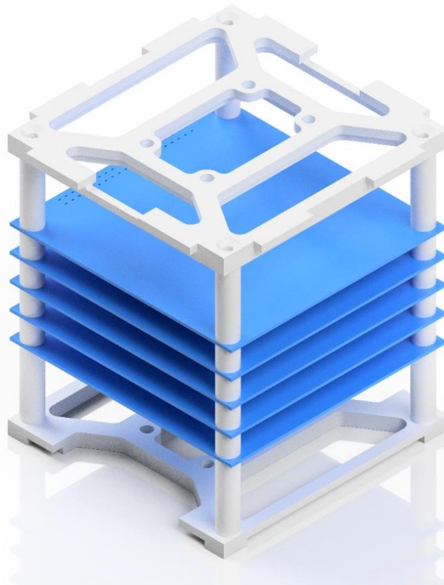
Figure 9 Example of PCB stack with correct spacing
