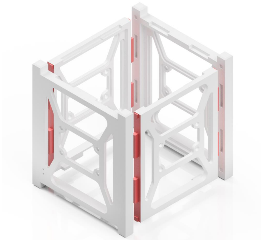
Figure 22 Sleeve glue up contact surfaces (red)
