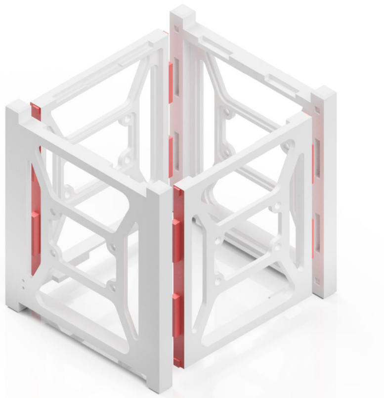
Figure 22 Sleeve glue up contact surfaces (red)
