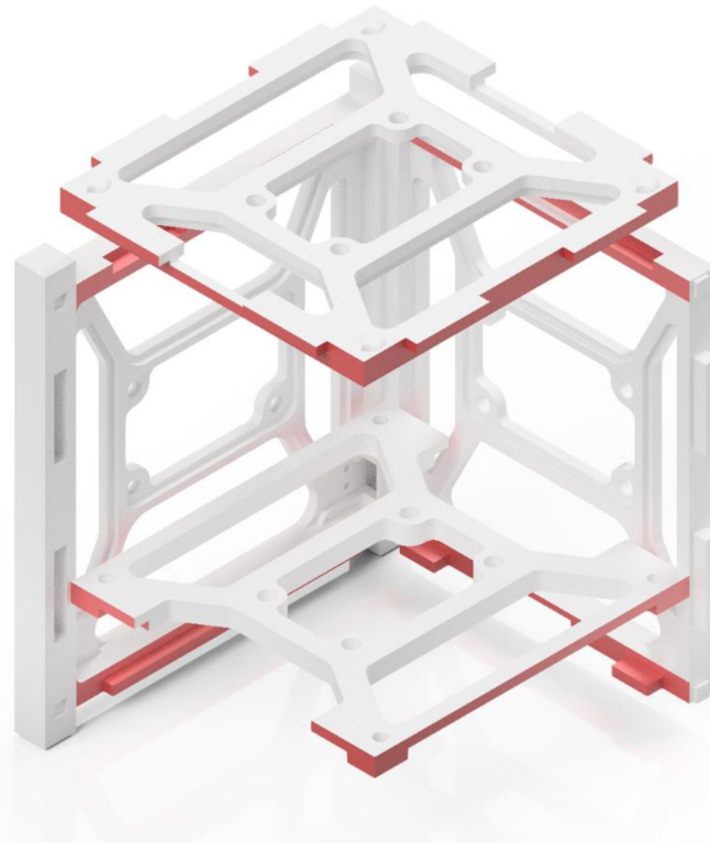
Figure 24 Glue up contact surfaces of the final assembly (red)
