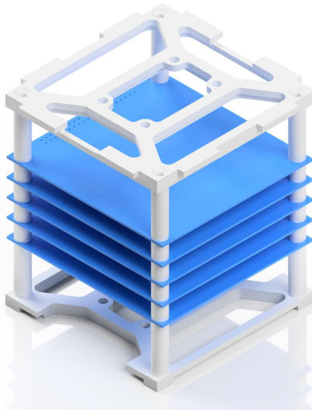
Figure 9 Example of PCB stack with correct spacing
