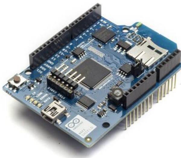
Obr. 6: Arduino Wi-Fi Shield [4]
