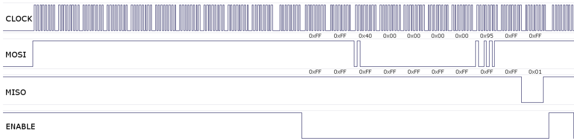
Figure 4.33: Waking up the card and setting the SPI mode
