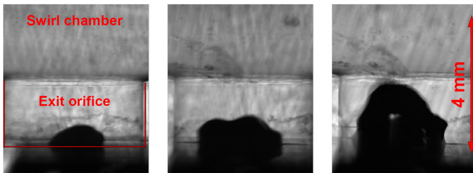
Fig. 7. The exit orifice in detail. SR atomizer, SFR 0, p-cymene, flow regime from left to right: equivalent to 0.5 MPa ( Re = 1075 ), equivalent to 1 MPa ( Re = 1431 ), equivalent to 1.5 MPa ( Re = 1731 ).
