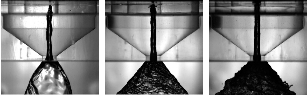
Figure 4 Typical results obtained from HS imaging. From left: Re = 1000, 2000 and 4000
