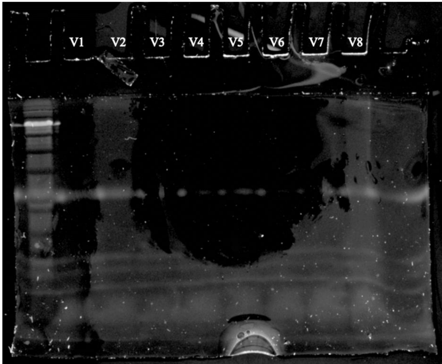
Figure 11: polyacrylamide gel produced with samples from a layer construction at pH = 9; V1 and V5 are negative controls with contamination. V1 – V4 have 4 base polyelectrolyte layers, V5 – V8 have 8 base polyelectrolyte layers. Each of these sequences has no enzyme and 0, 2, or 4 covering layers above the enzyme respectively. TCE stained and analyzed under UV light.
