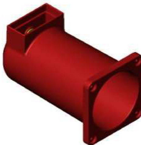
Obr. 5: Epoxidová komora [CAD]
