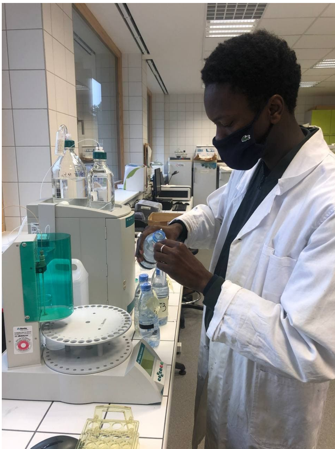
Figure 4.12: Student Ing. Doudou BA, performing ionic chromatograph analysis at the laboratory of Prof.Vymazal of the Faculty of Environmental Sciences, CZU, Prague 2021
