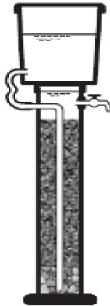
Figure 3.10: Stratified column of brick chips, pebbles and coconut shells as used in Sri Lanka.
