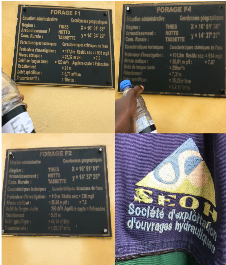
Figure 4.5: Geographic coordinates and technical characteristics of boreholes
