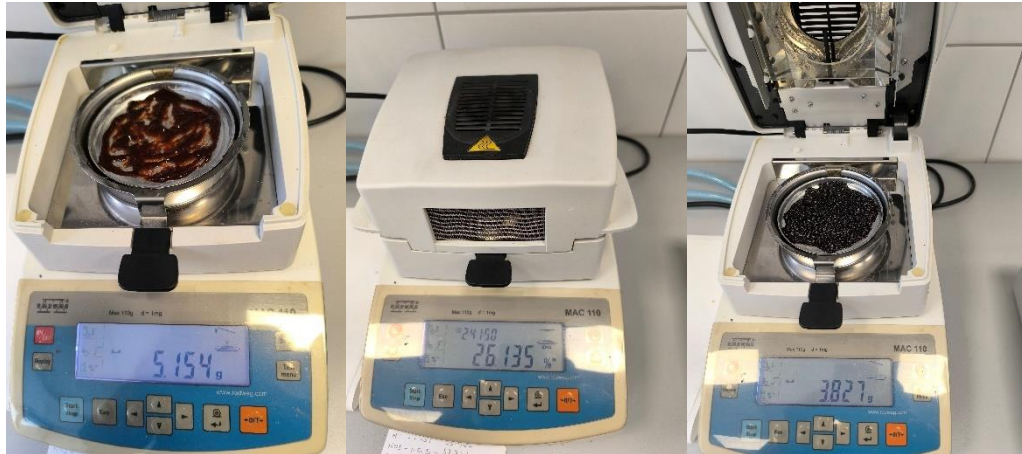
Figure 7: Apparatus (RADWAG MAC 110) used for the analysis of moisture content.
