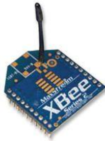
Obr. 4.1: Modul XBee Series 2
