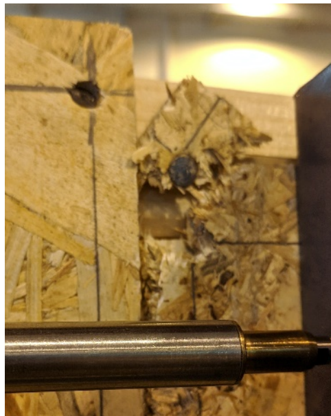
Figure 5.5 – Failure of the corner fasteners
