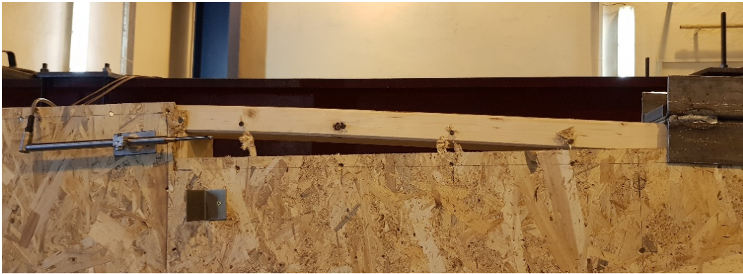
Figure 5.6 – Groups fastener failure (unzipping) of nails in the top rail
