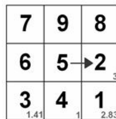
Figure 3-8(Bartak, 2009) The SFD8 algorithm. The large numbers denote the elevations, the small numbers denote the slope from the central cell, and the arrow represents the determined flow direction.
