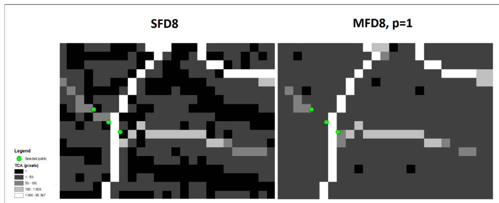
Figure 5-31 Example of great differences in TCA by MFD and SFD near water streams (white)
