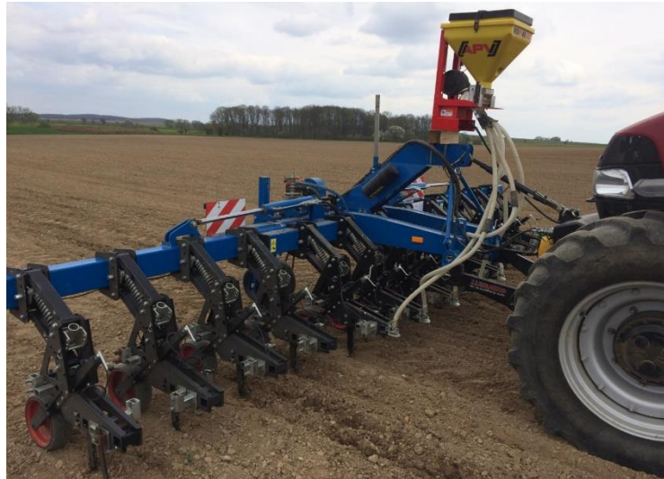
Figure 44 Establishing a sugar beet stand with the simultaneous sowing of spraying rows (photo by Kroulík).
