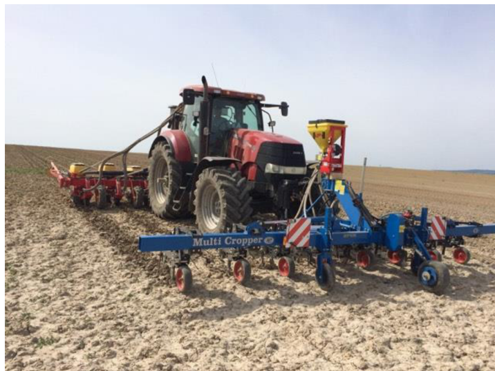
Figure 40 Establishing a maize stand with the simultaneous sowing of spraying rows (photo by Kroulík).
