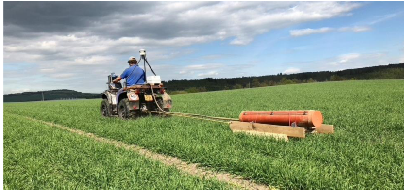
Figure 18 Measurement of electrical conductivity of the soil with the EM38MK2 probe.
