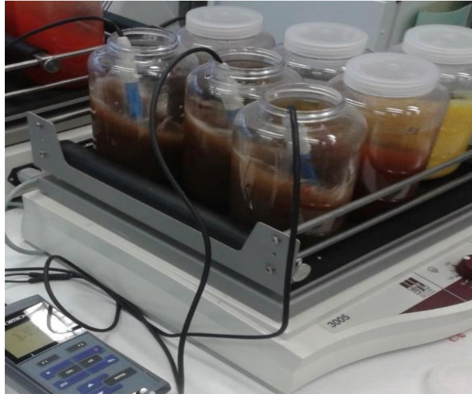
Figure 11. Photo of an orbital shaker (model GFL 3005).
