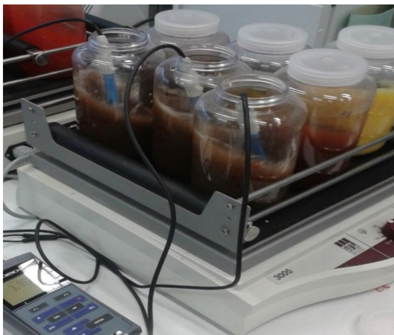
Figure 11. Suspensions are shaking using an orbital shaker (model GFL 3005).
