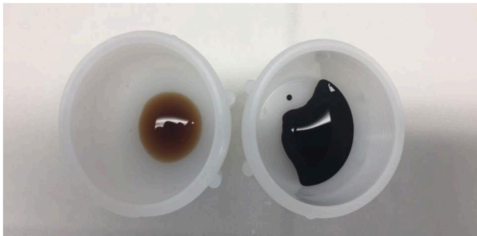
Figure 13. Decomposition of humic acids with 2% nitric acid. pH = 4 (left), pH = 6.5 - 9 (right).
