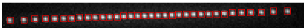
Figure 3.9: The image of the 34\ ^{40}\text{Ca}^+ ion string taken by EMCCD camera during the measurement. The red squares represent borders of the areas used to process and evaluate whether the selected ion is bright or dark.
