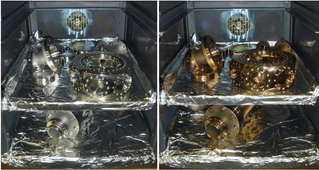
Figure 3.2: Stainless steel parts inside the oven. On the left before air-bake, on the right after the air-bake.
