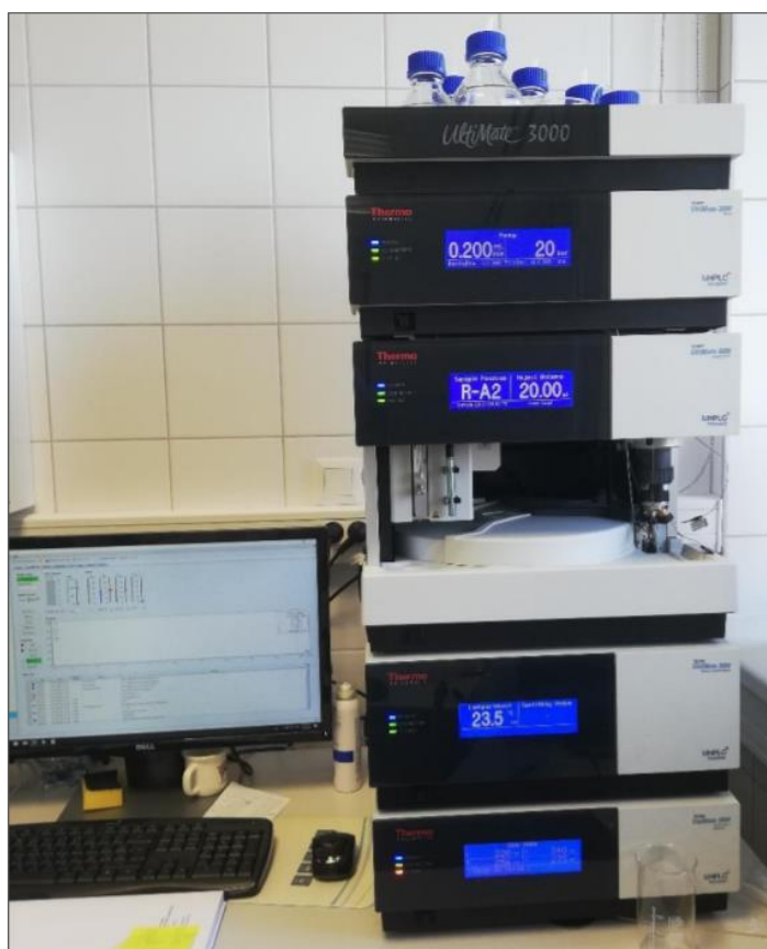
Figure 9: HPLC combined with Thermo Scientific™ Dionex™ Ultimate™ 3000
