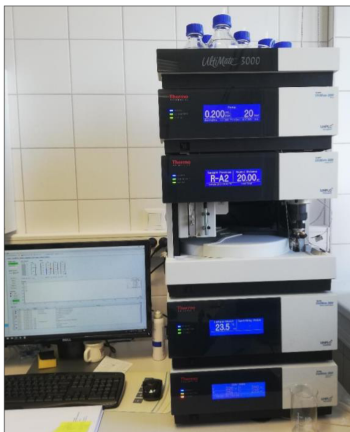
Figure 9: HPLC combined with Thermo Scientific™ Dionex™ Ultimate™ 3000
