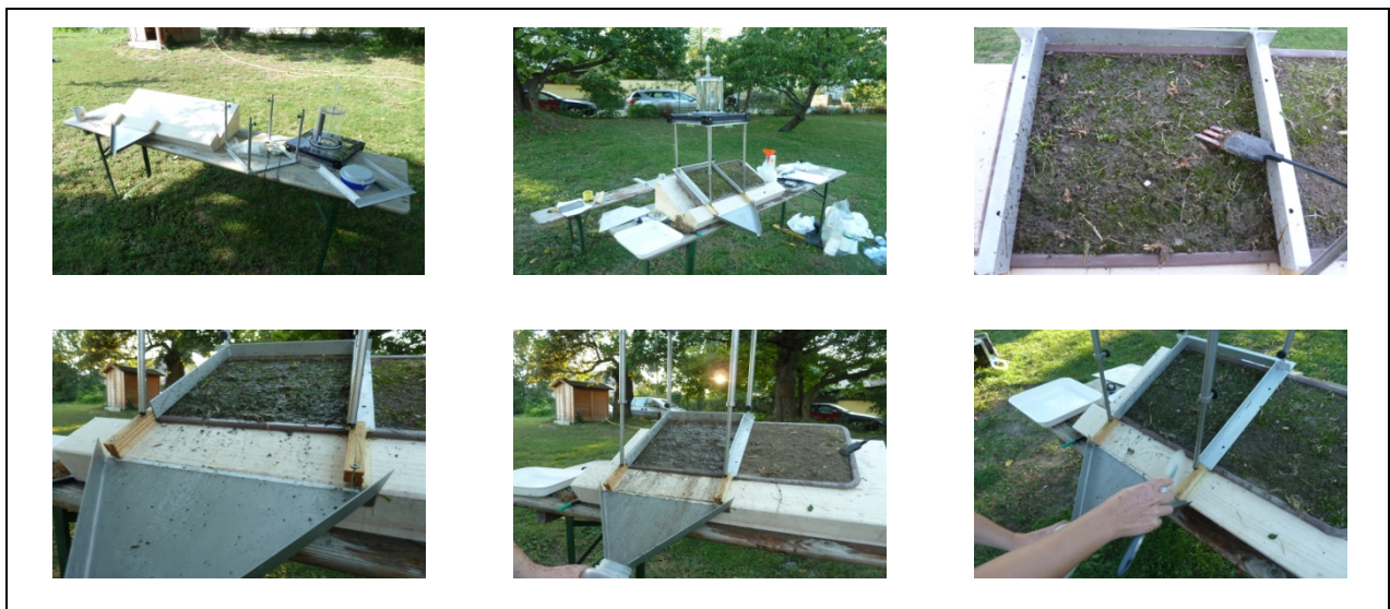
Figure 19 Working steps of implementation of rainfall simulation (18.09.2012 Essling, VIENNA)
