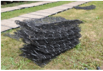
Figure 9 MacMat ® R geotextile – turf reinforcement mat (TRM) (15.05.2012, Essling VIENNA)
