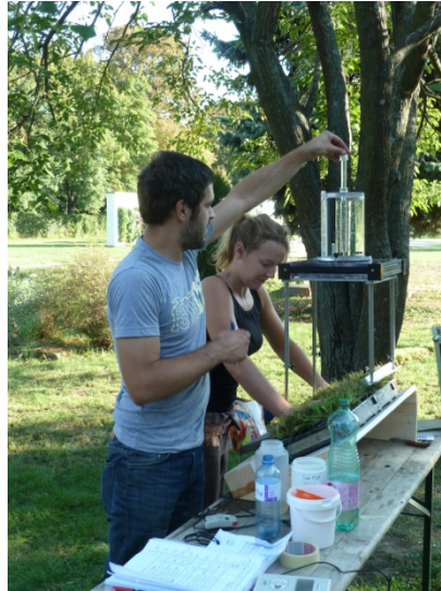
Figure 18 Rainfall simulation (18.09.2012 Essling, VIENNA)
