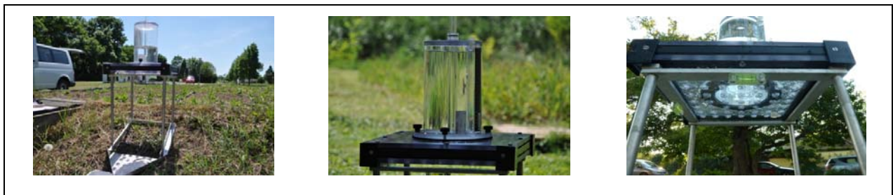
Figure 5 Rainfall simulator (09.05.2012, Essling, VIENNA)
