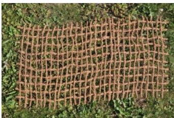
Figure 10 BonTerra ® Coir Netting (15.05.2012, Essling VIENNA)
