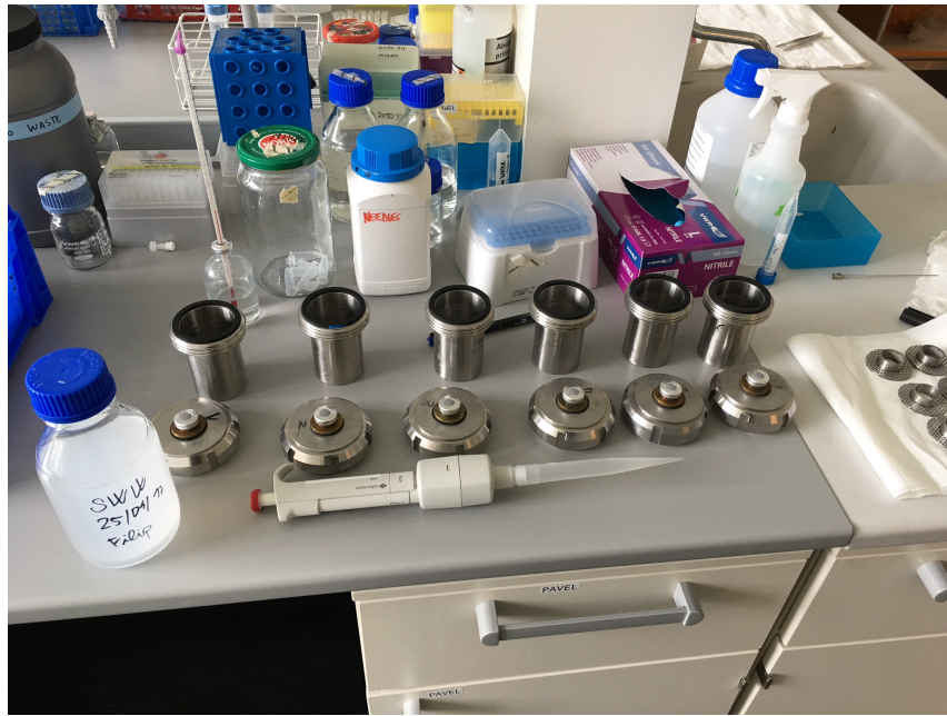
Figure B2: Stainless steel gas-tight reactors for biofilm testing.
