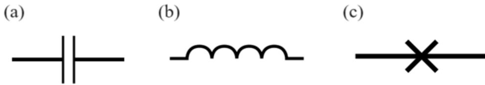
Figure 1.1: Three circuit elements. (a) Circuit symbolism for a linear capacitor -  $C$ . (b) Circuit symbolism for a linear inductor -  $L$ . (c) Circuit symbolism for a non-linear Josephson junction -  $E_J$  and  $C_J$ .
