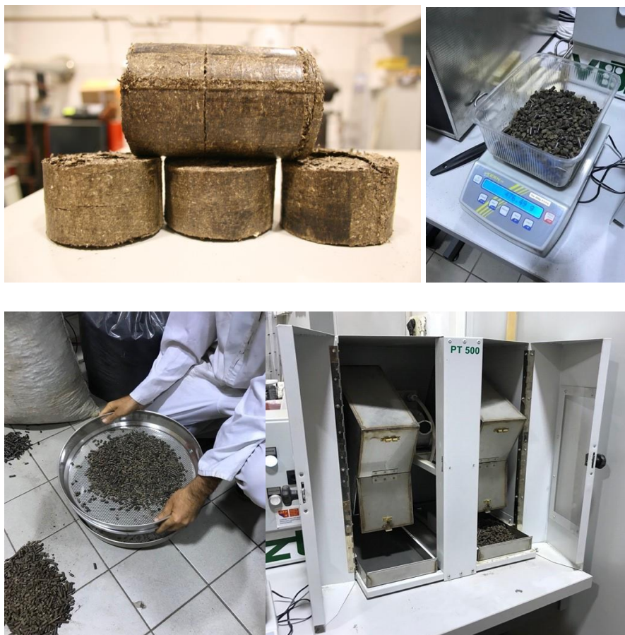
Figure 29 Pellets durability testing and Po briquette samples
