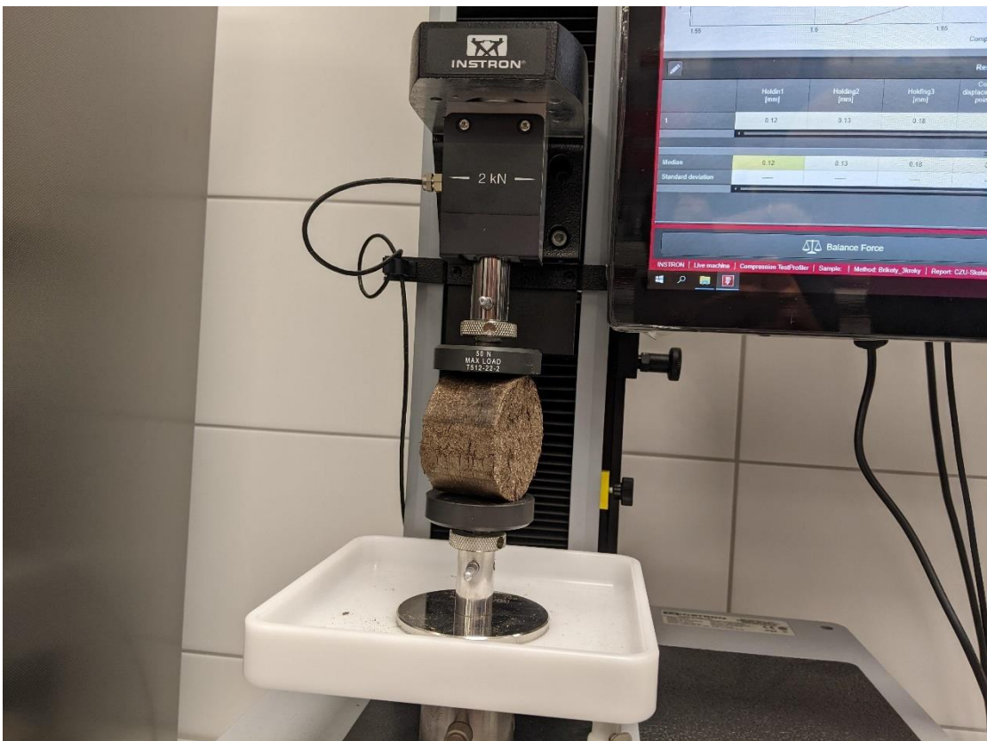
Figure 8. Mechanical durability testing of ZoCy briquettes
