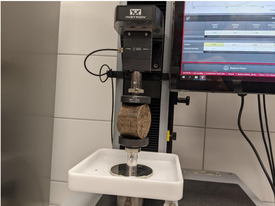
Figure 8. Mechanical durability testing of ZoCy briquettes
