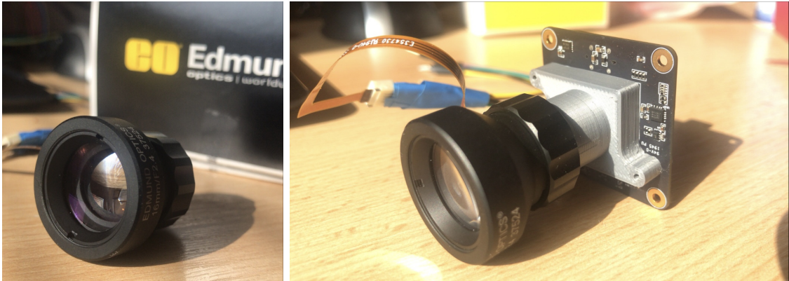
Figure 3.1: The lens is sold either as an individual component or along with a mount system. The first picture shows the lens with a mount system and the second image shows the lens mounted onto a camera.
