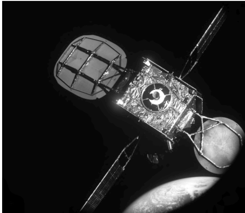
Figure 3.1: View of IS-901 satellite from MEV-1 „near hold“ position during approach (figure courtesy [20])
