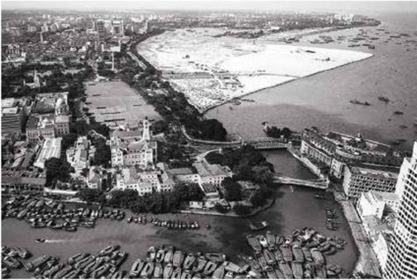
Figure 16-Seven phases of the East Coast Reclamation, which started in 1966 and lasted for around 30 years, resulted into the creation of Marina Bay in the early 2000's. (© Urban Redevelopment Authority. All rights reserved.)
