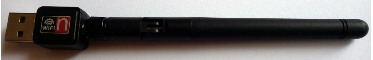
Pic. [7] WiFi dongle with external antenna
