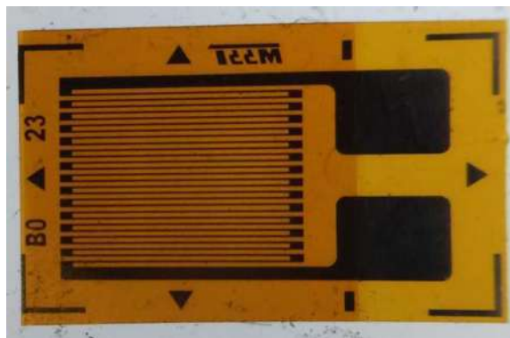
Figure 2.5: Strain gauge. Relative positions of conductive paths change the conductance of the sensor and hence allow for a strain response of attached surface detection. The image is taken from Wikipedia 3 .
