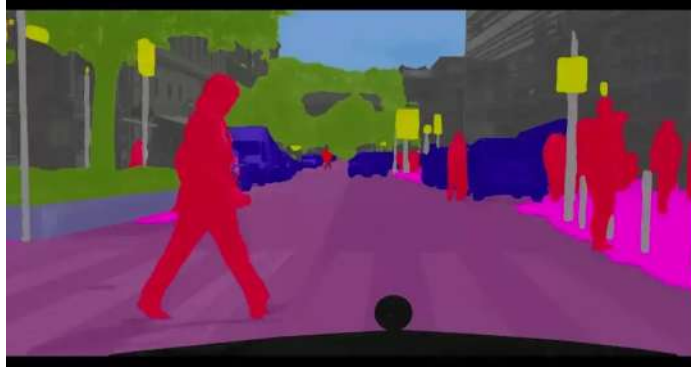
Figure 2.3: An example of image segmentation. Every class of object (e.g. person, road, and traffic sign) is coloured by its assigned colour. Image taken from Kanan [14].
