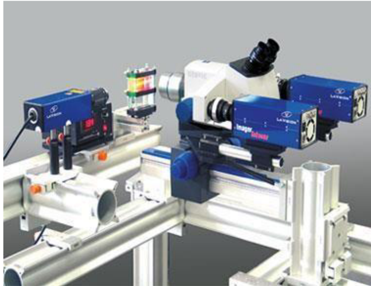
Figure 7: Micro PIV setup [22]
