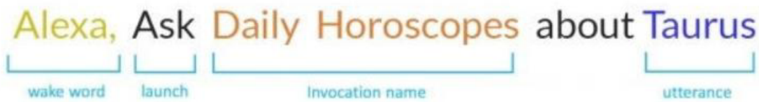
Figure 5: Example of an “order” using Amazon Alexa. Voice assistant listens for a wake word, which is followed by information containing a specific skill with the addition of intent. Retrieved from [47].
