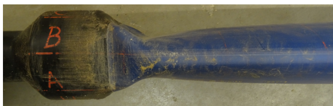
Obr. 14.104 Deformace potrubí - detail (vzorek C-D110-SDR17-BV-1)
