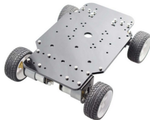
(b) 4WD Ackerman Steering RC Car [22]
