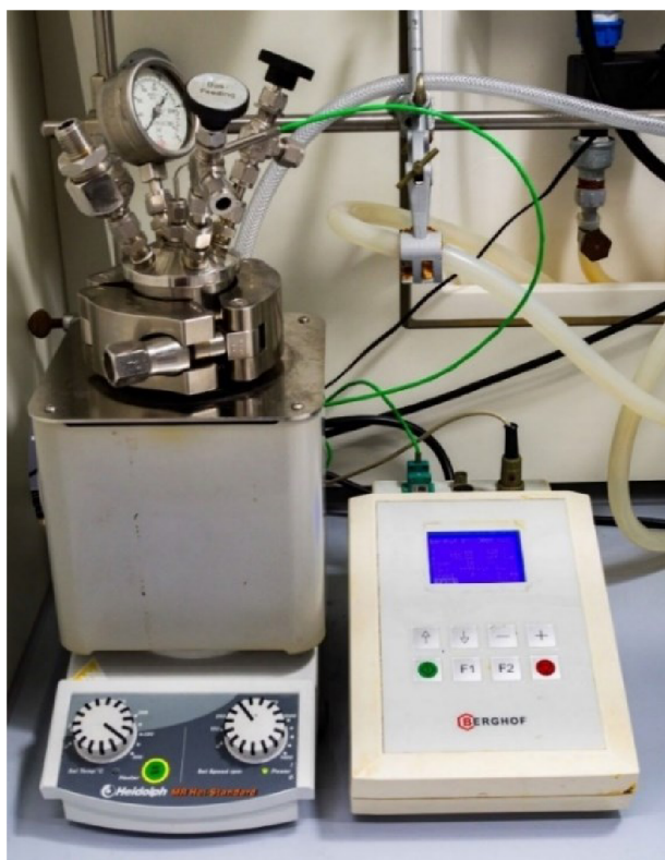
Figure 10: The hydrothermal reactor with heating and stirring plate is shown on the left side, the thermostat control unit for the reactor is depicted on the right side.
