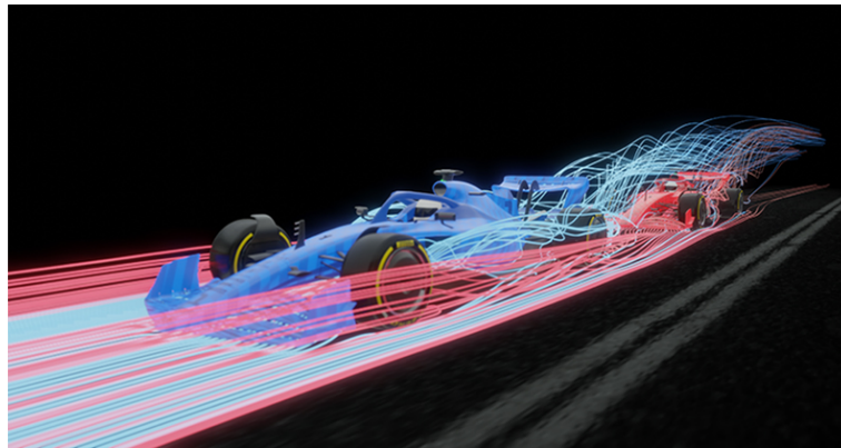
Figure 1.1: Result of a CFD simulation showing streamlines around an F1 car
