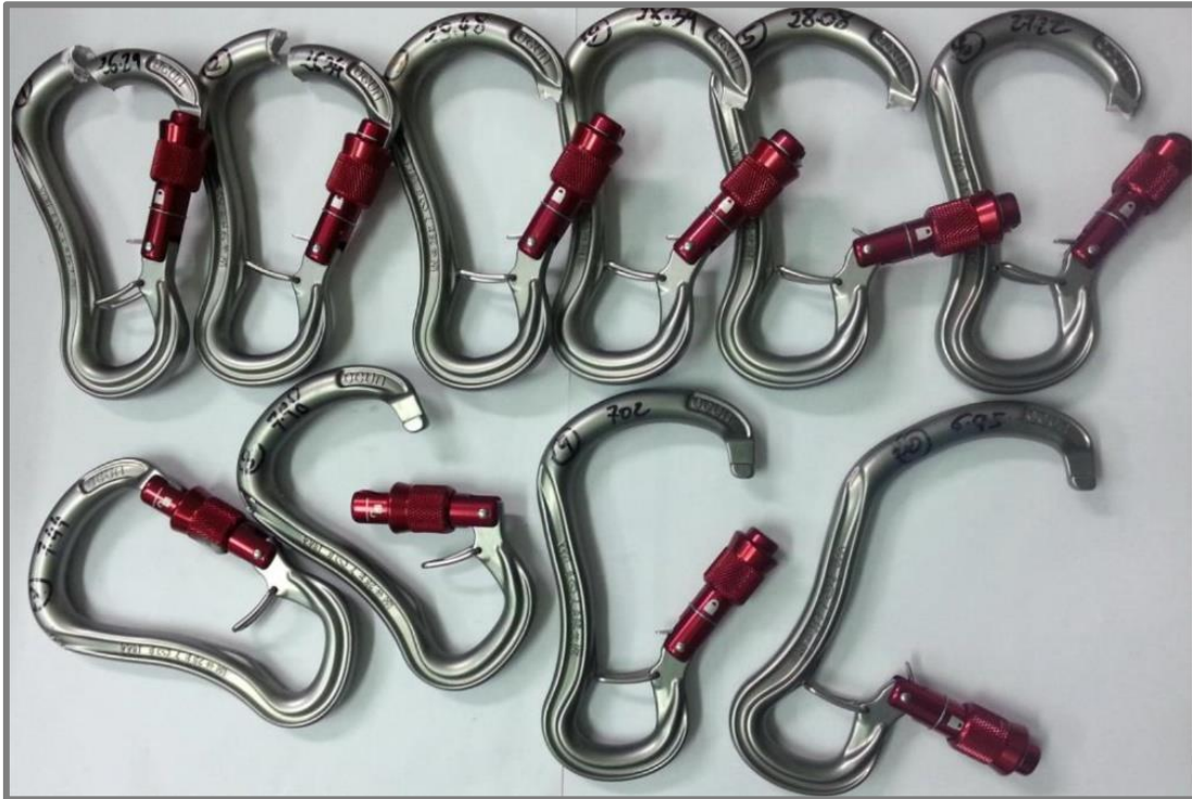
Obr. 4-26 Deformace karabiny Condor (23)
