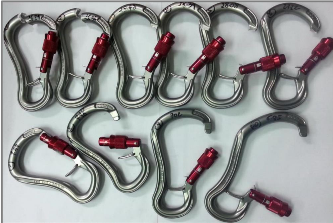
Obr. 4-26 Deformace karabiny Condor (23)
