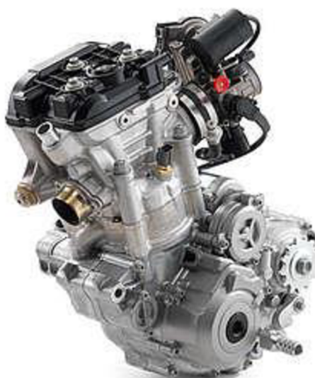
Obr. 2 Motor KTM 250 SX-F 2014 [2]
