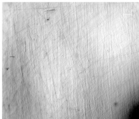
Fig. 3.12: Optical image of the CdTe surface before any etching – surface grooves caused by the lapping are clearly visible.
