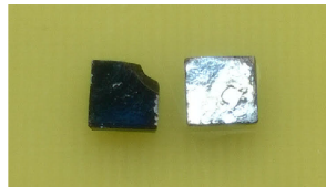
Fig. 3.1: CdTe samples after being etched in the solution used for (111)A and (111)B identification. (111)A side (left) is matt, (111)B side (right) becomes bright.
