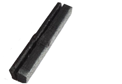
Figure 3.11 Interlaminar failure of specimen 2
