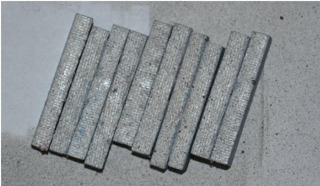
Figure 2.3 Random texture on the SBS specimen [21]
