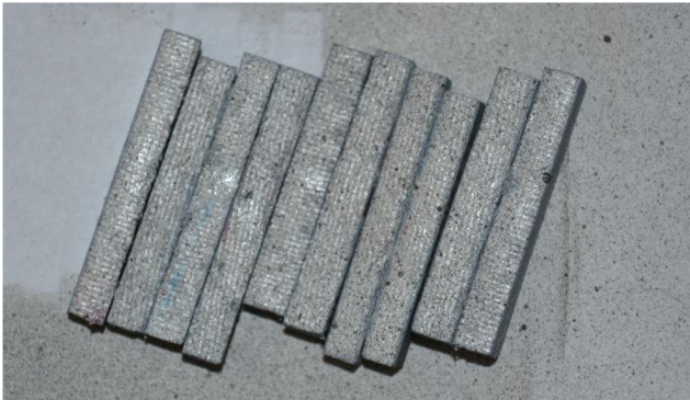
Figure 2.3 Random texture on the SBS specimen [21]
