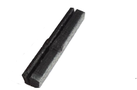
Figure 3.11 Interlaminar failure of specimen 2
