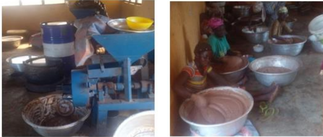
Figure 4: Electric milling (left) machine and processors kneading milled kernels with hands (right) (Source: Field observations).
