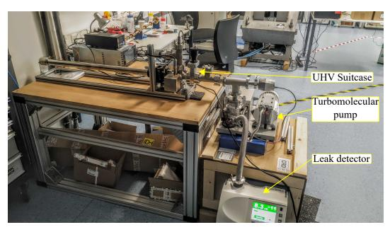
**Figure 6.3:** UHV suitcase connected to the turbomolecular pump with a pre-pumping leak detector. Some leaks contained in the chamber were detected using this detector.
