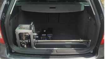
**Figure 6.10:** (a) UHV suitcase during the transport to the car trunk. (b) UHV Suitcase in the car trunk. The ion pump controller and UPS can also be seen, which has to be connected to the UHV suitcase to avoid pressure decreasing during transport.
