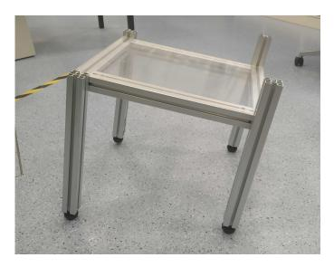
**Figure A.3:** Support system consists of aluminium profiles. At the end of the each leg, there is an adjustable screw leg for easy adjustment.
