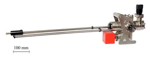
**Figure 5.5:** Small and compact UHV suitcase from company Scienta Omicron uses wobblestick as a linear transport.
