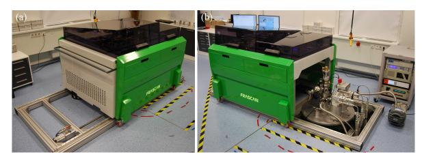
**Figure 2.5:** A newly-built HF-EPR spectrometer in CEITEC Nano MOTeS laboratory. (a) In the measurement position. (b) In the waveguide loading position.
