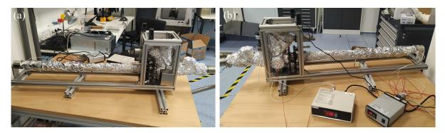
**Figure A.4:** View of the baking procedure of the UHV suitcase. The entire suitcase is wrapped with baking tapes and heated up to 120°C. Temperature was controlled by two controllers showed in (b).
