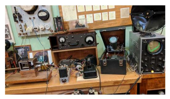
**Figure 2.1:** Experimental setup of the first EPR measurement made by Zavoisky in 1944. Photographed and provided author's friend Dennis Schäfter at the Zavoisky Museum Lab, Kazan Federal University, Russia.
