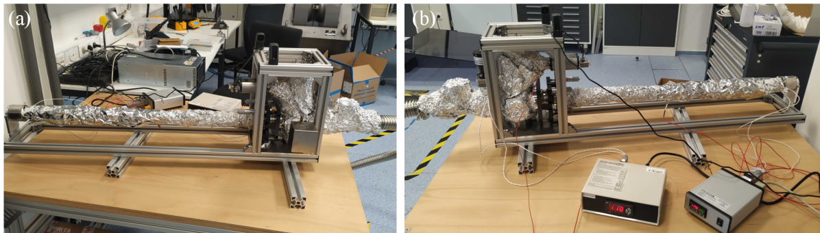
Figure A.4: View of the baking procedure of the UHV suitcase. The entire suitcase is wrapped with baking tapes and heated up to 120°C. Temperature was controlled by two controllers showed in (b).
