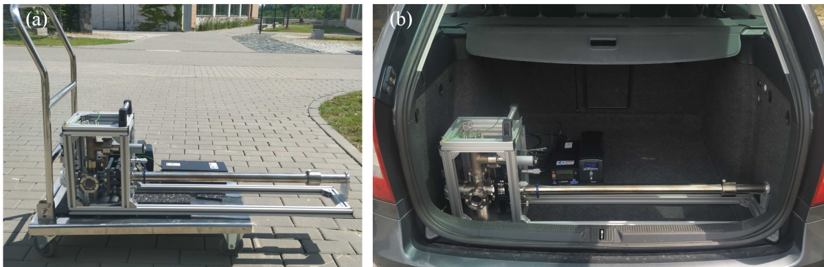
Figure 6.10: (a) UHV suitcase during the transport to the car trunk. (b) UHV Suitcase in the car trunk. The ion pump controller and UPS can also be seen, which has to be connected to the UHV suitcase to avoid pressure decreasing during transport.
