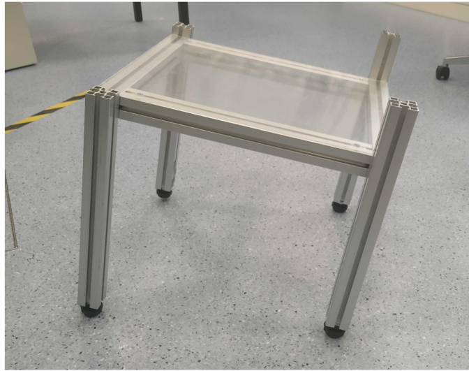
Figure A.3: Support system consists of aluminium profiles. At the end of the each leg, there is an adjustable screw leg for easy adjustment.
