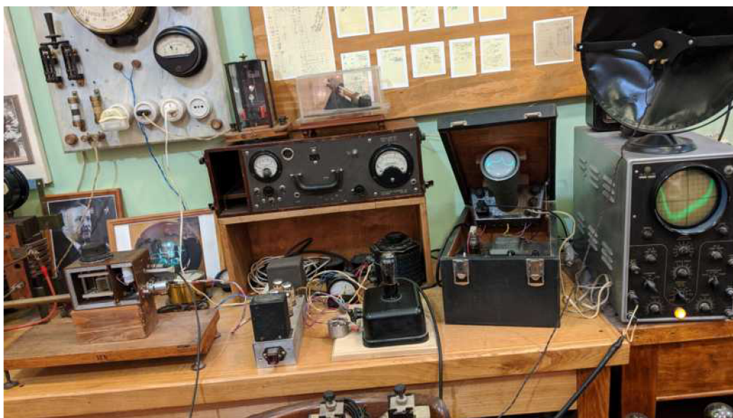
Figure 2.1: Experimental setup of the first EPR measurement made by Zavoisky in 1944. Photographed and provided author's friend Dennis Schäfer at the Zavoisky Museum Lab, Kazan Federal University, Russia.
