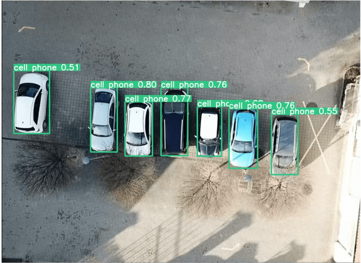
Figure 6.4: Cars are detected incorrectly as cell phones when the source image is taken from a top-down view.
